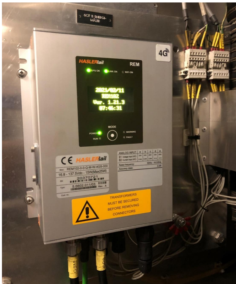
Example of an energy measurement unit installed in a locomotive
